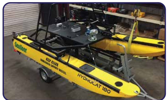
HydroCat-180 can be easily transported via trailer
